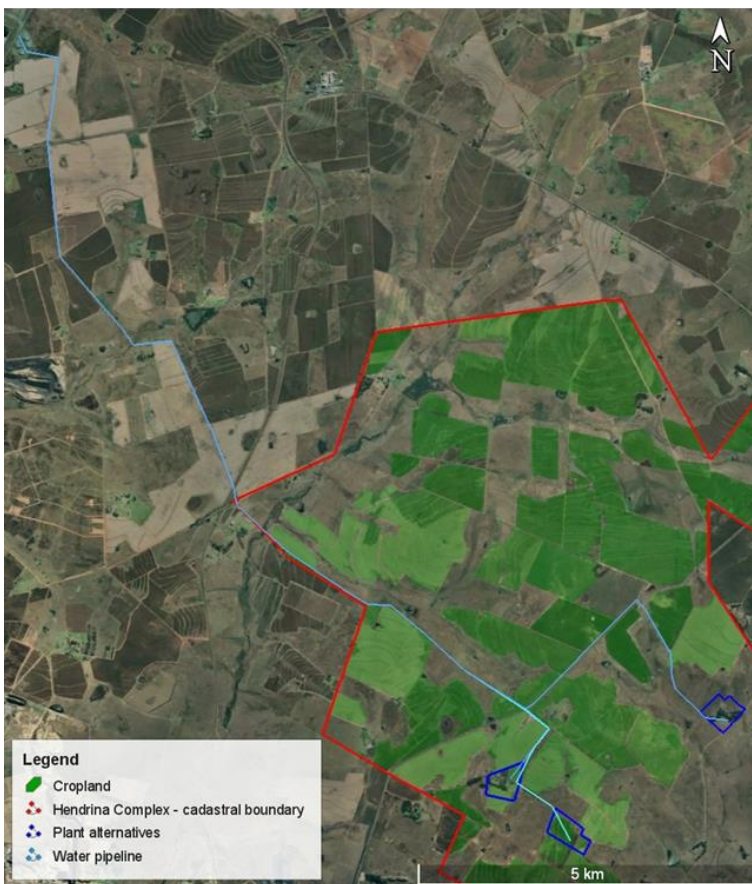
Figure 7-11: Satellite image map of the proposed pipelines to the alternative facility sites.
