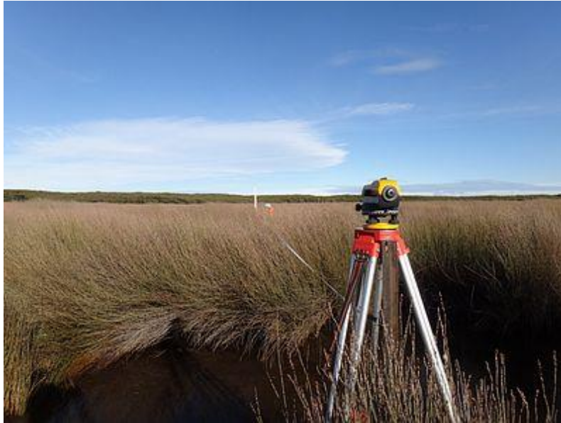
Photo 2: Using the builder's level to measure changes in elevation along T11_2012 (Bythell, 2012)
