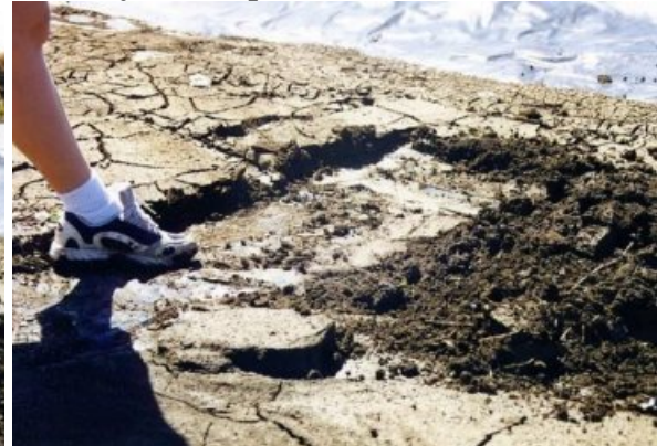
Sediment trapped upslope of Vetiver filter strips
