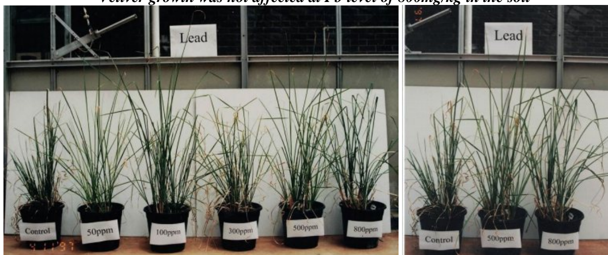
Vetiver growth was not affected at Pb level of 800mg/kg in the soil
