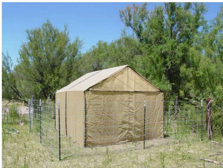
Figure 12. ARS peaked-roof 10 x 12 x 6-8 (h) ft \frac{3}{4} " EMT conduit field cage (note livestock/wildlife fence).
