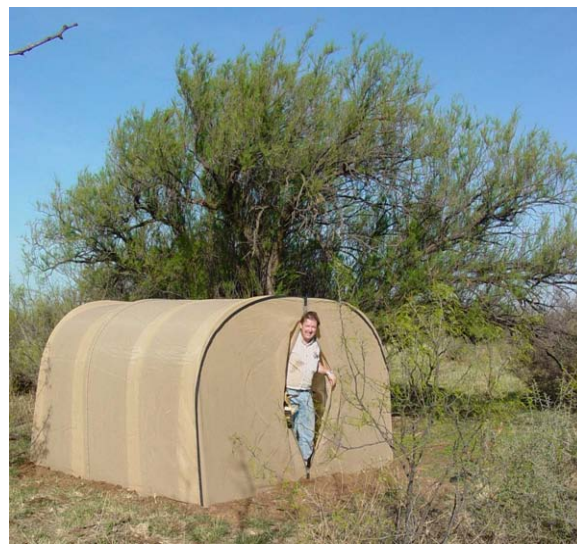
Figure 13. AgriLife arched-top 1 5/8" SS20 piping field cage used in releases at the Murphy Ranch and at Buzzards Draw.
