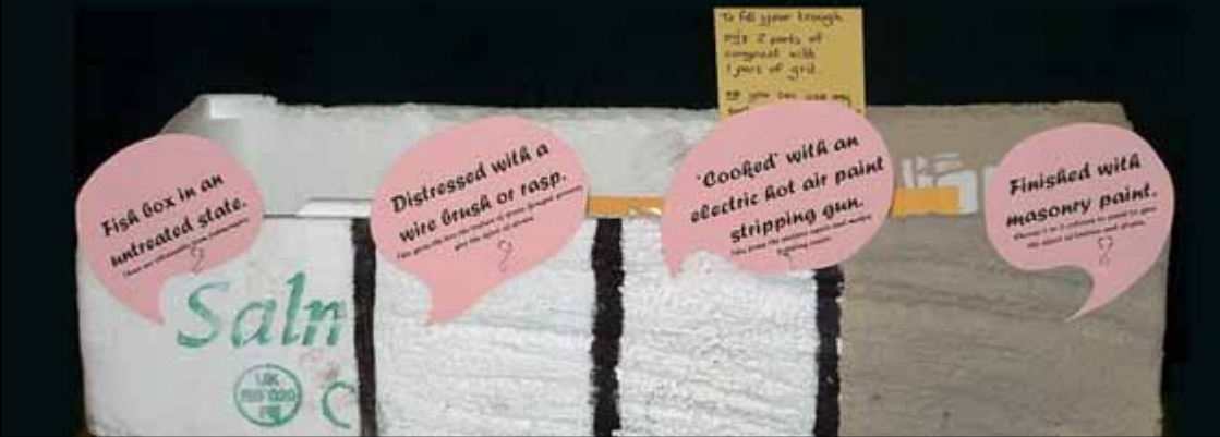
99 - Construction of a fish-box trough
