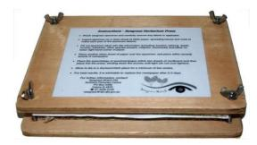
The press should be exposed to a gentle heat source, avoiding excessive heat that will "cook" the specimens. Sometimes it is possible to use the heat from the sun. In this case the presses should be small. If fire is the heat source, keep the press at a safe distance to prevent fire starting on the press.
