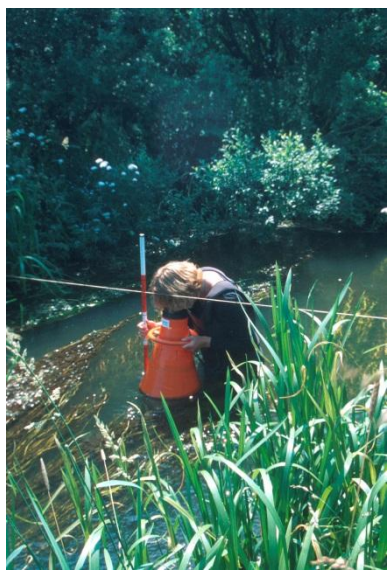
Figure 3.4 Survey of macrophyte vegetation in a Danish stream. According to the Danish Monitoring Programme, macrophyte recordings are made in approximately 250 plots (25 x 25 cm) in each stream reach placed adjacently along 10 cross-sectional transects.
