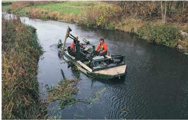
Figure 3.5 Weed cutting in a middle-sized Danish stream. The vegetation is cut close to the stream bottom from razors mounted on the boat.
