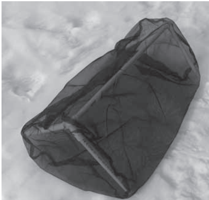
FIG. 1. PVC pipe frame and mesh bag for sampling clutch size. Images are courtesy of Barbara Doyle and Billy Barr.
