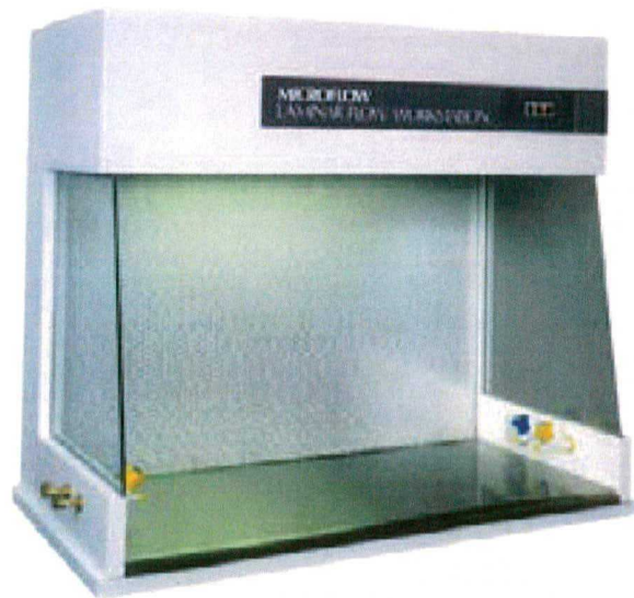
Figure 2 A commercial laminar flow work station Often called a "hood".
