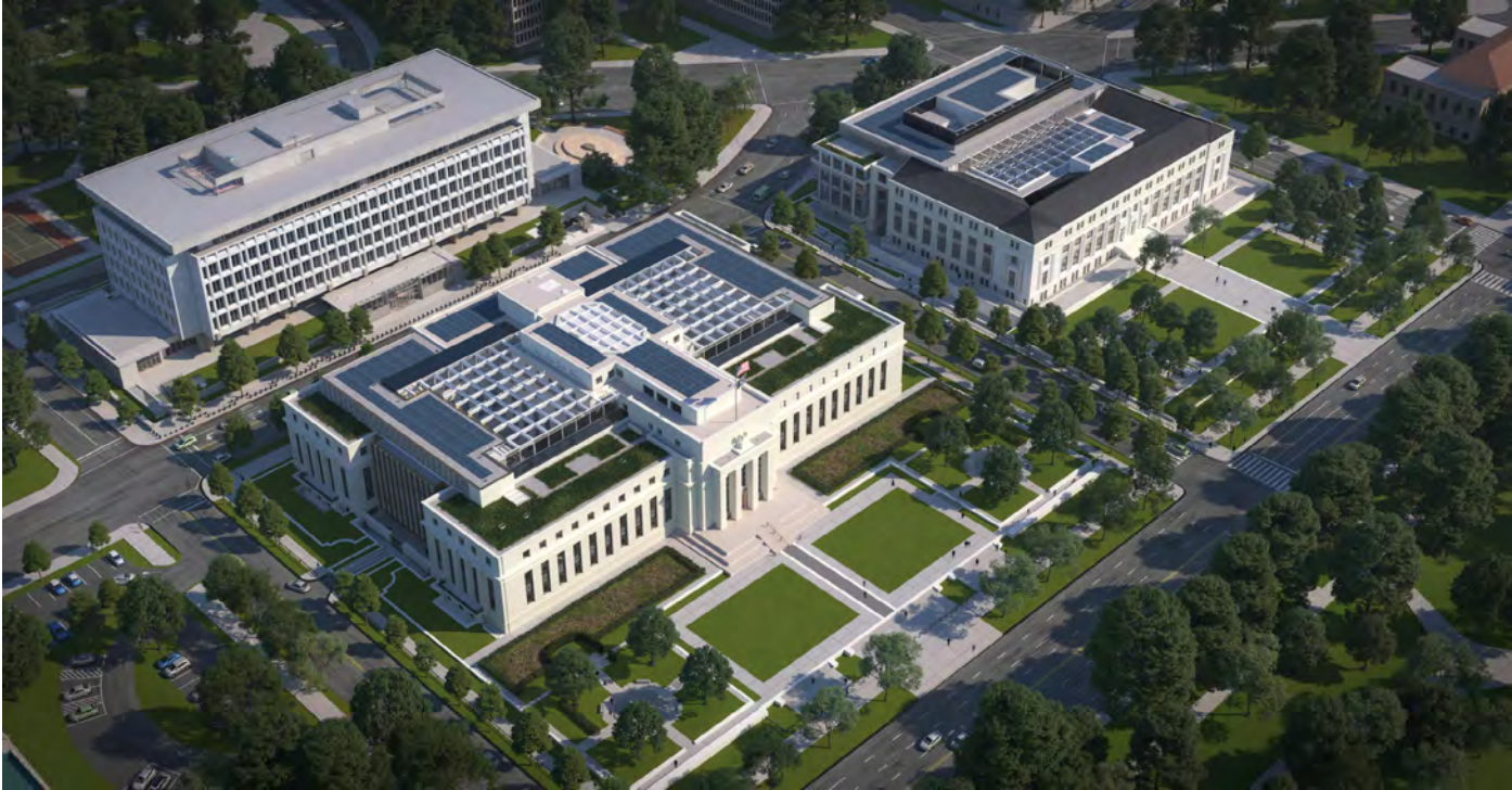
Figure 2.10: View of Eccles (left) and FRB-East (right) showing proposed skylights and roof systems.
