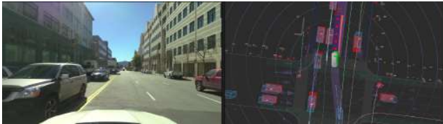
Fig. 6. SafetyNet failure case in simulation. Two simultaneous situations - SDV driving close to dividing line, and a sudden velocity change of the oncoming vehicle - combine to reveal a limitation in the implementation.
