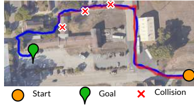
Figure 6: GPS-Nav (red) fails to execute a plan due to its inability to reason about traversability through obstacles, while LM-Nav (blue) succeeds.
