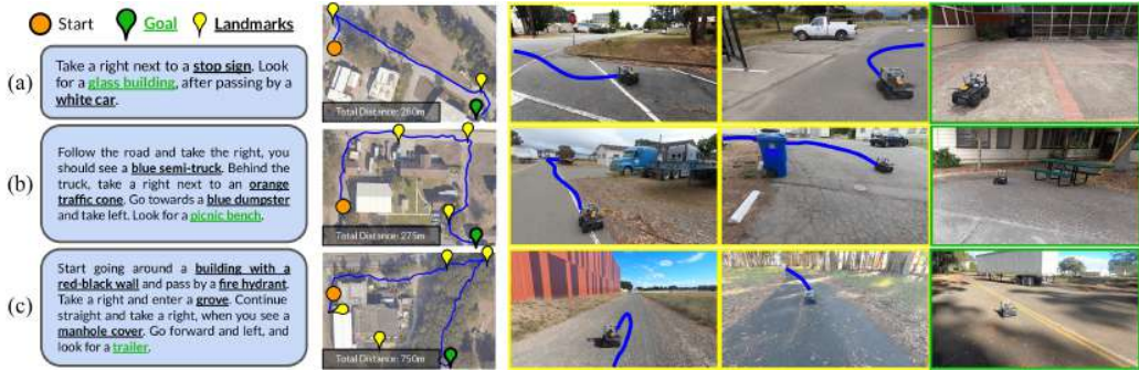
Figure 4: Qualitative examples of LM-Nav in real-world environments executing textual instructions (left). The landmarks extracted by LLM (highlighted in text) are grounded into visual observations by VLM (center; overhead image not available to the robot). The resulting walk of the graph is executed by VNM (right).
