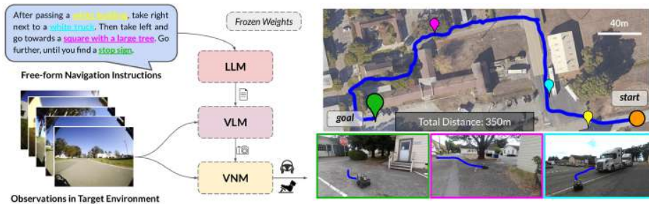
Figure 1: Embodied instruction following with LM-Nav: Our system takes as input a set of raw observations from the target environment and free-form textual instructions (left), deriving an actionable plan using three pre-trained models: a large language model (LLM) for extracting landmarks, a vision-and-language model (VLM) for grounding, and a visual navigation model (VNM) for execution. This enables LM-Nav to follow textual instructions in complex environments purely from visual observations (right) without any fine-tuning .
