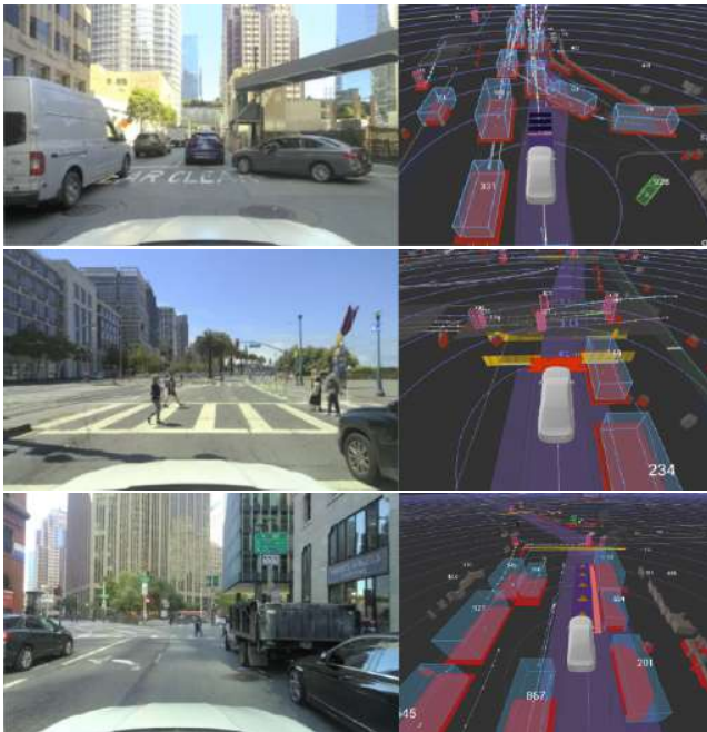
Fig. 7. Examples of successful ML planner behavior (no fallback trajectory was triggered) in the real world. Top : merging, middle : yielding to pedestrians, and bottom : nudging around a parked car.
