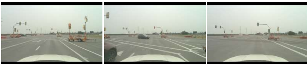
Figure 5: Front-camera footage of our planner stopping for a red light, and subsequently crossing the intersection when the signal turns green (images from left to right, recorded several seconds apart).
