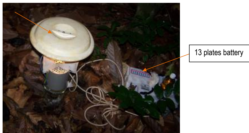
Plate 3: The Pirbright light trap (arrowed) used for insect sampling.
