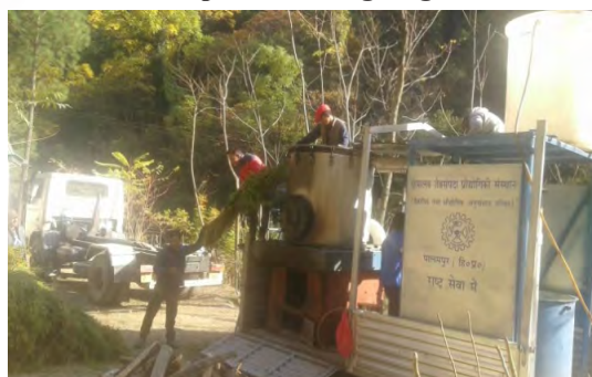
Mobile distillation unit
