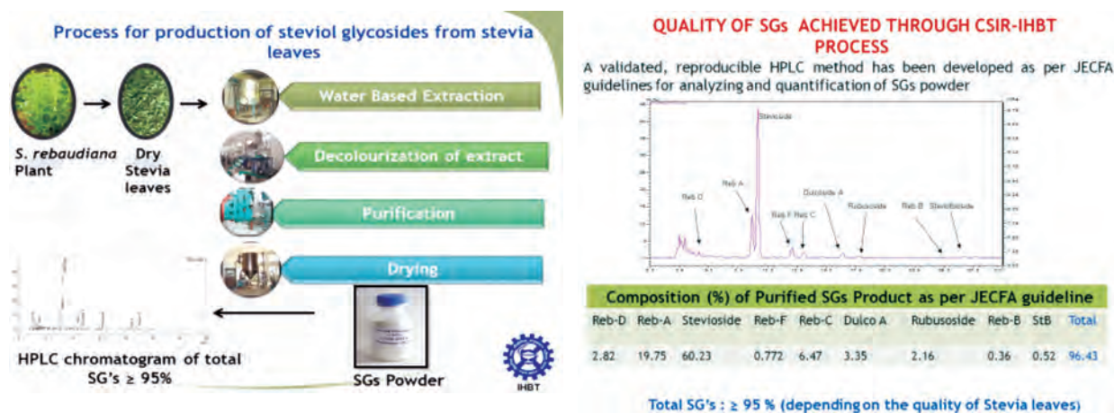
Fig. 14 Process for upscaling of steviol glycosides up to 50 kg/batch
