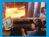
Rotek Incorporated offers a wide selection of seamless rolled rings in aluminum grades, and in carbon, stainless and alloy steels. All are certified, all are traceable. Rings can be produced in diameters from 18 inches to 160 inches, heights to 20 inches and weights to 8,000 pounds. Available profile configurations range from simple rectangular cross sections to complex shapes, including flanges, grooves and tapers.
