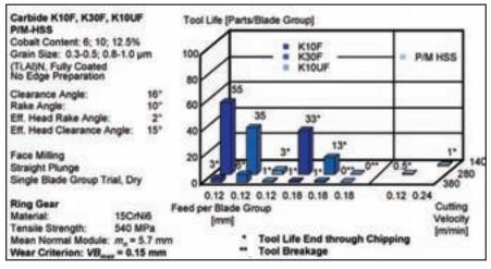
Figure 8—Tool life overview of the substrate variation.
