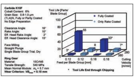
Figure 12—Tool life comparison between fully coated tools and only-rake-coated tools.
