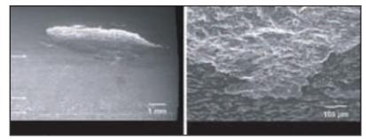
Figure 4—SEM images of the No. 10 tooth of the tested pinion gear of the LH2 run using 7.5 cSt oil with an FZG Type GF-C micropitting gear. The area between the two outer arrows is the micropitting band.
