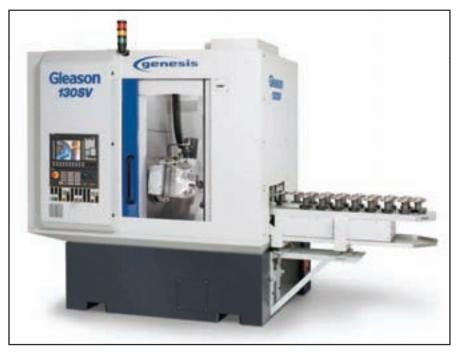
customer is that he gets a fully capable machine to do all the shaving technologies, like plunge and diagonal shaving."
