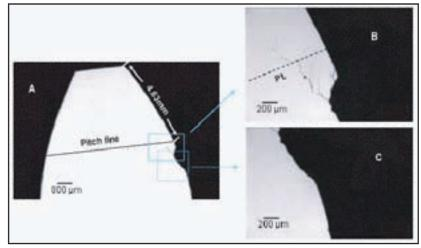
Figure 6—SEM image of a cross section through a spall on the 9th tooth of the HL3 run. This test involves a 15 cSt oil and a pitting gear.
