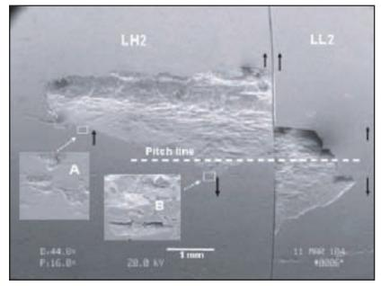
Figure 8—Micropitting crack directions before and after pitch line on the micropitting gear (LH2). The SEM was taken together from the two pinions. The location of the pitch line is defined with respect to the LH2 pinion; it is only approximate for the LL2 pinion. The magnification for the insert is 300X.
