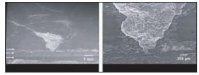
Figure 2—SEM images of the No. 5 tooth of tested pinion gear of the LL2 run using the 7.5 cSt oil with an FZG Type PT-C pitting gear. The area between the two outer arrows is the micropitting band.
