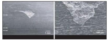
Figure 3—SEM images of the No. 2 tooth of the tested pinion gear of the HH2 run using 15 cSt oil with an FZG Type GF-C micropitting gear. The area between the two outer arrows is the micropitting band.
