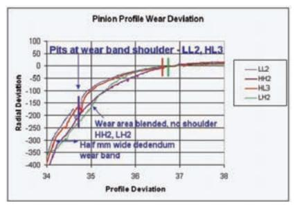
Figure 5—Wear-induced tooth profile deviation.
