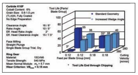
Figure 13—Wear charts of the only-rake-coated tools.
