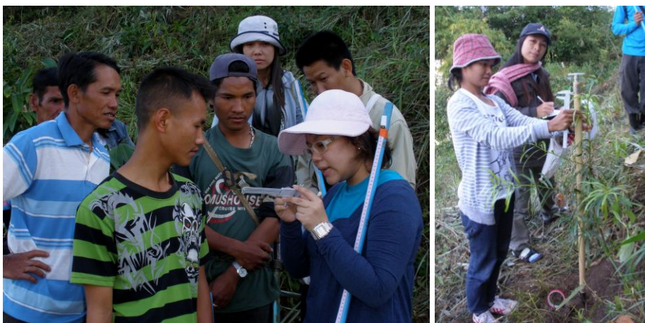
Far left: teaching Ban Lo Yo villagers how to use Vernier callipers to measure root collar diameter. Left: Measuring a Podo-carpus tree.
