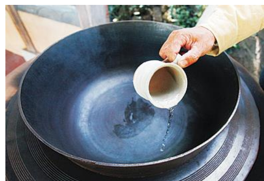
Photo 40. Measuring the caldron's temperature by dropping water
