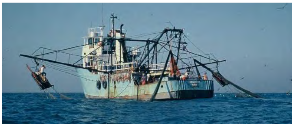
Figure 5.15 Photograph of a typical crustacean trawl vessel.
