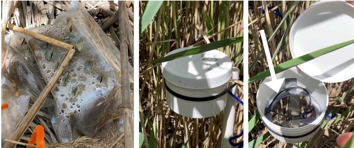
Fig. 40. Leftover floral foam blocks used to hold cut Phragmites stems inoculated with Archanara spp. larvae (left; note slits in plastic to hold individual Phragmites stems). Closed (middle) and open (right) egg release containers. Containers are closed in the field to protect against predation. However, the open container on the right illustrates the nested container design—eggs were placed into a PVC cup with an open top (missing in this photo), which was held inside of the larger container by the black ziptie (shown by white arrow). Once larvae emerged from eggs, they climbed over the top of the inner PVC cup, then fell through the mesh bottom of the outer cup into the Phragmites stand.
