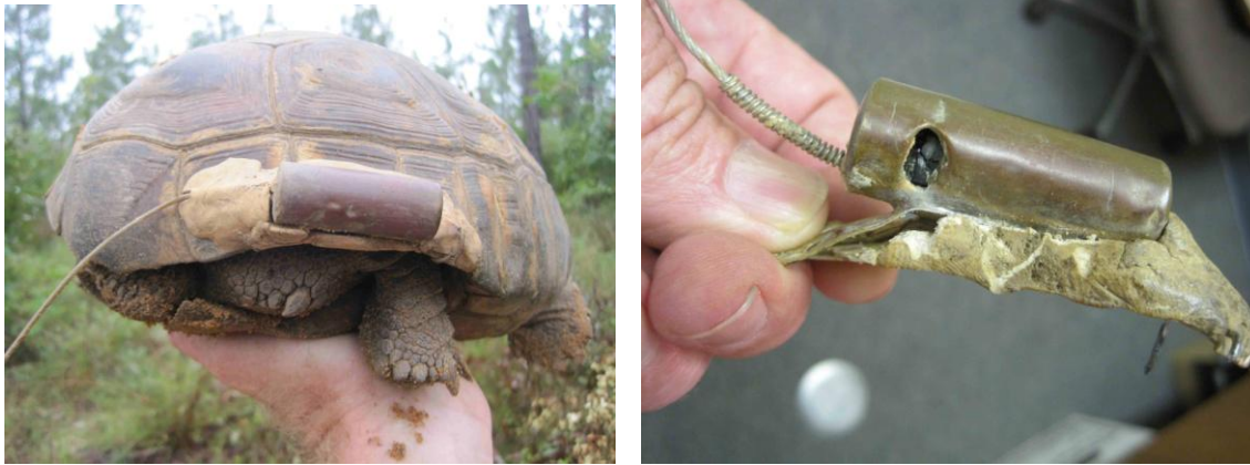
Figure 2. One of the radio-tracked tortoises with damage to its radio from dog bites, but the radio was still attached and the tortoise seemed fine (left). A radio recovered by the burrow of tortoise #100 after dogs ripped the radio off of the tortoise and ruined the radio; the tortoise is OK (right).
