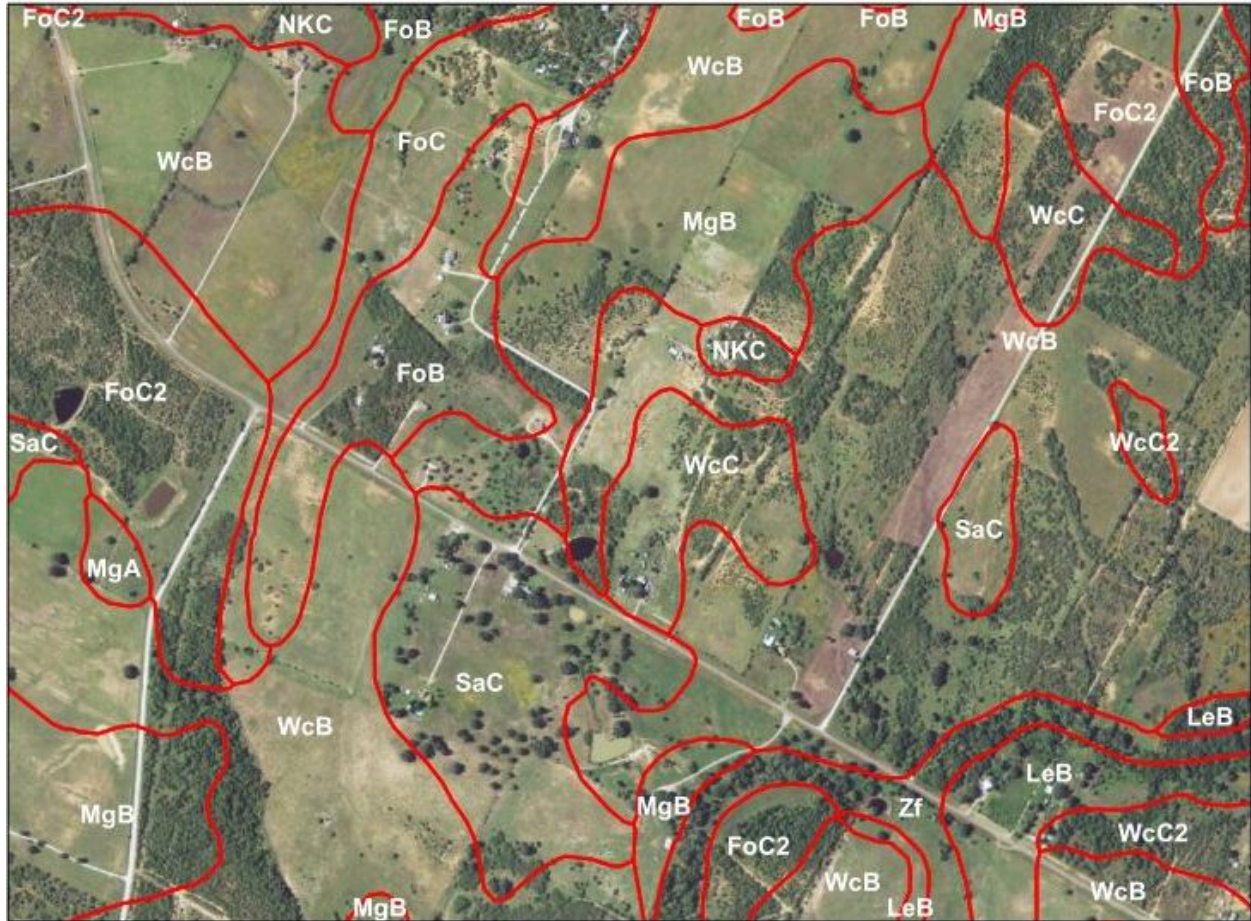
Figure 5.1 Example of the spatial distribution of NRCS soil units on a portion of the Wilson County landscape.
