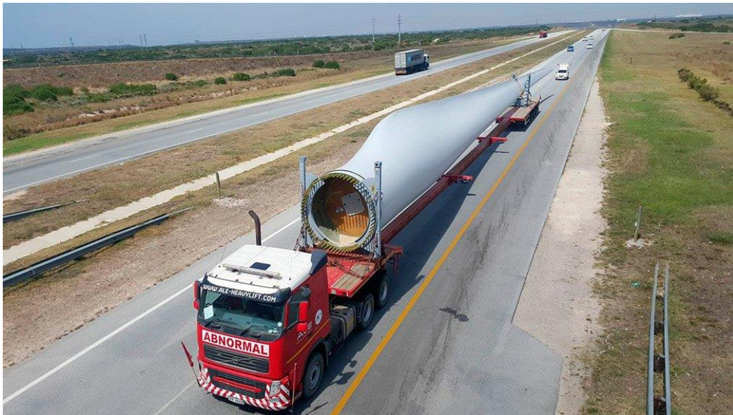
Figure 2.11: Example of a wind turbine blade being transported on an extendible trailer (Source: Google Images, 2021)
