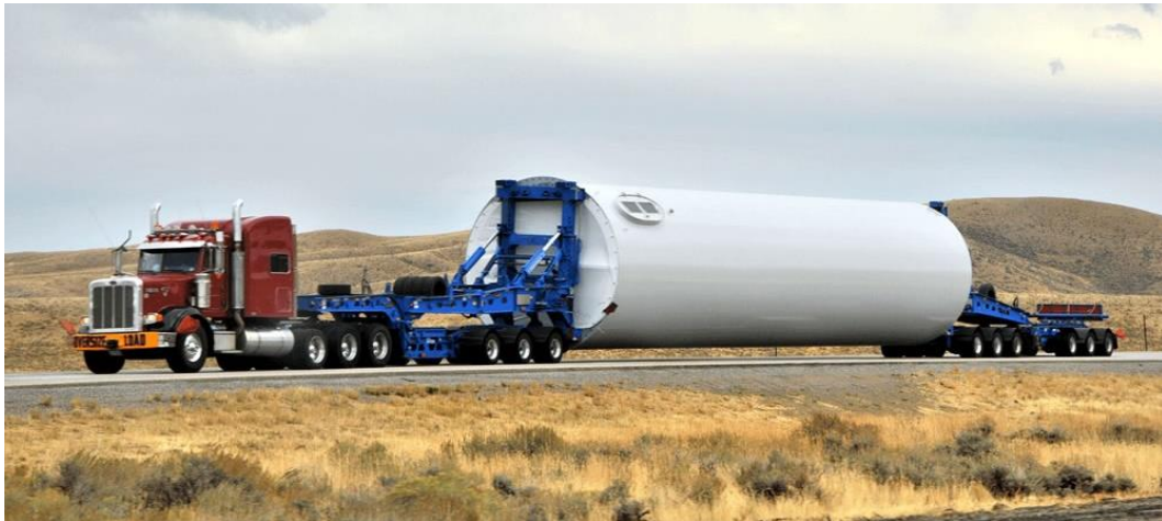
Figure 2.10: Example of a tower section being transported (Source: Google Images, 2021)
