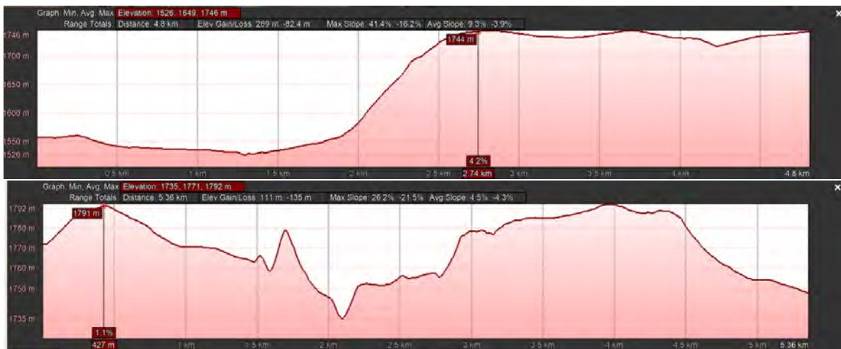
Figure 3.2: Elevation profile of (a) the north-western half of the proposed OHL and (b) the south-eastern half of the proposed OHL.
