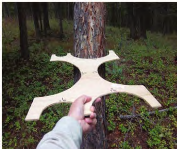
Figure 6. displaying how to classify CWD in each diameter class using the go or no go gauge.
