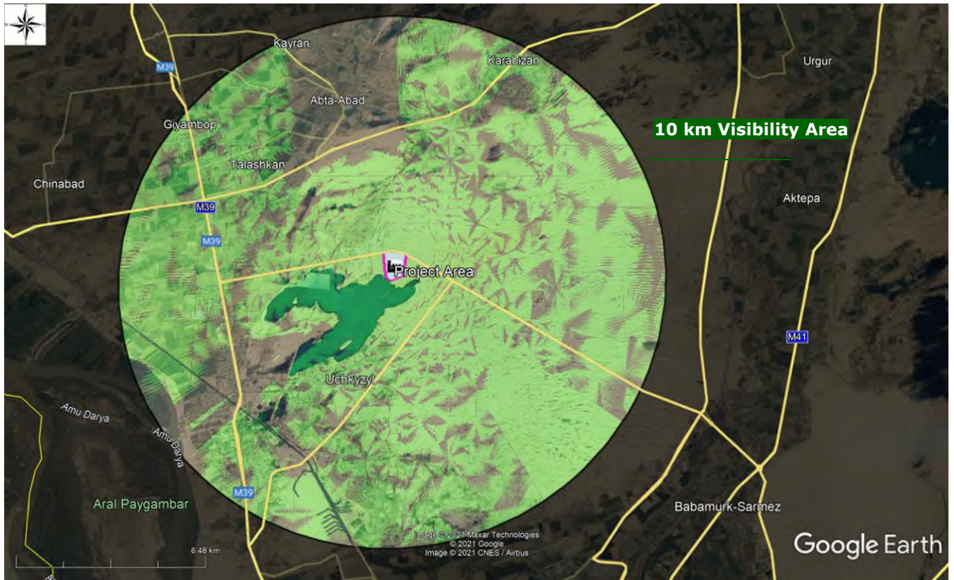
Figure 108: Project Area visibility within the 10 km radius area (Project Area can be seen from the green shaded areas)
