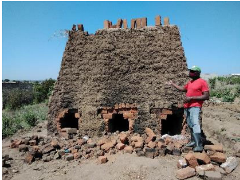
Block production furnace, Vila Nova
