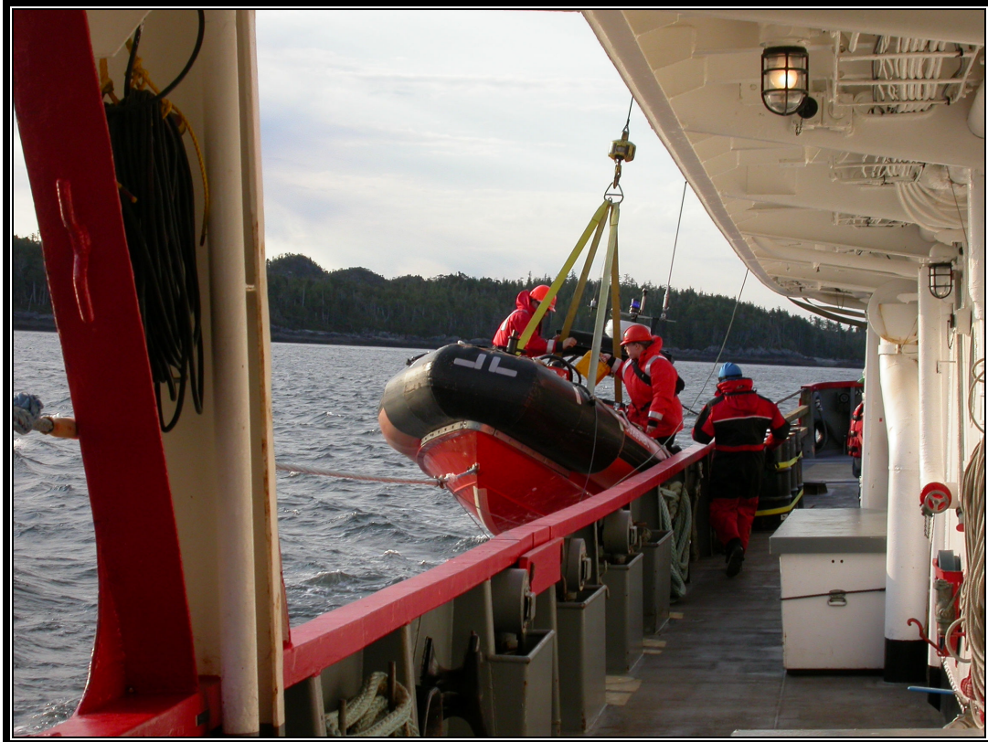
Zodiac 640 being deployed to recover an oceanographic buoy
