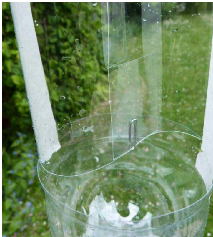
Figure 13: Detail of the aerial interception trap, showing the internal surface of the trap.
