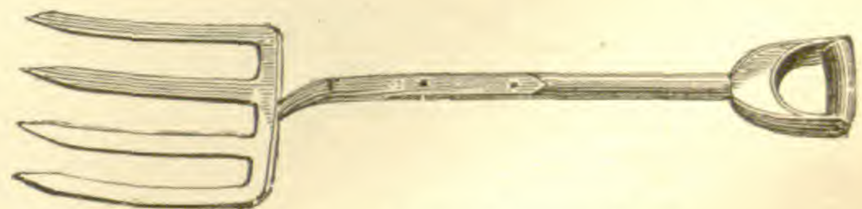
FIG. 22. FLAT-TINED DIGGING FORK.
