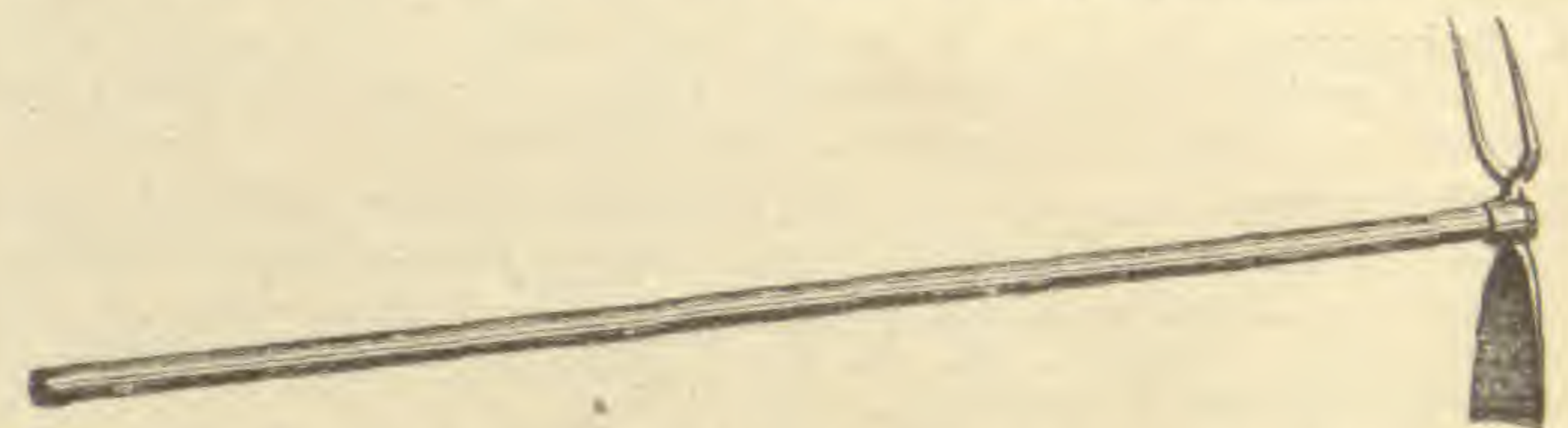
FIG. 235. DRAW HOE AND FORK COMBINED.
