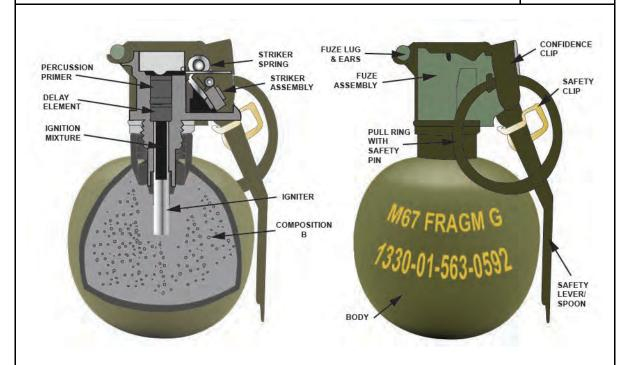
Note. M67 hand grenades developed before 2009 are not fitted with confidence clips (CCs).
