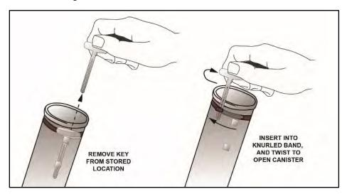
Figure B-8. Handheld signal individual sealed steel container
