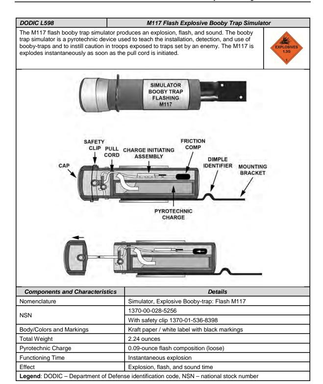
Figure 4-11. M117 flash explosive booby trap simulator
