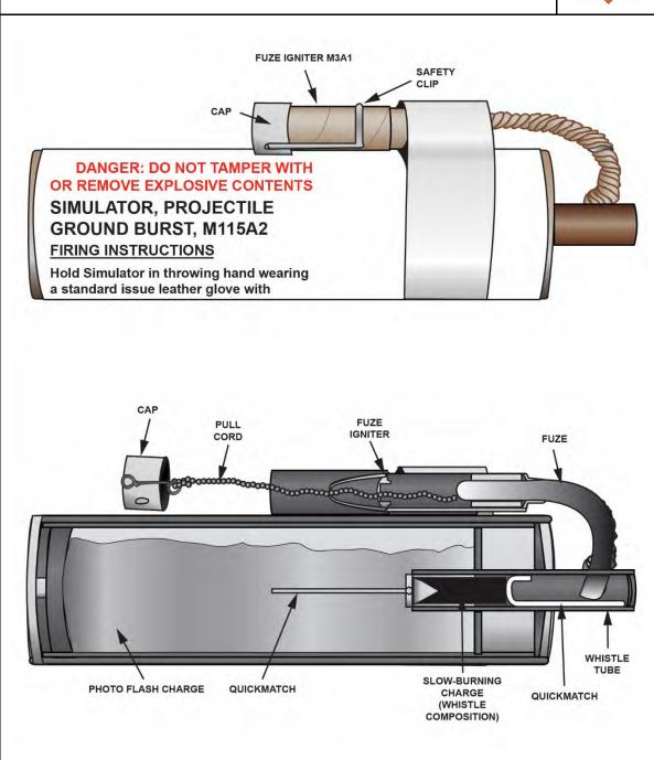
Figure 4-15. M115A2 ground burst simulator
