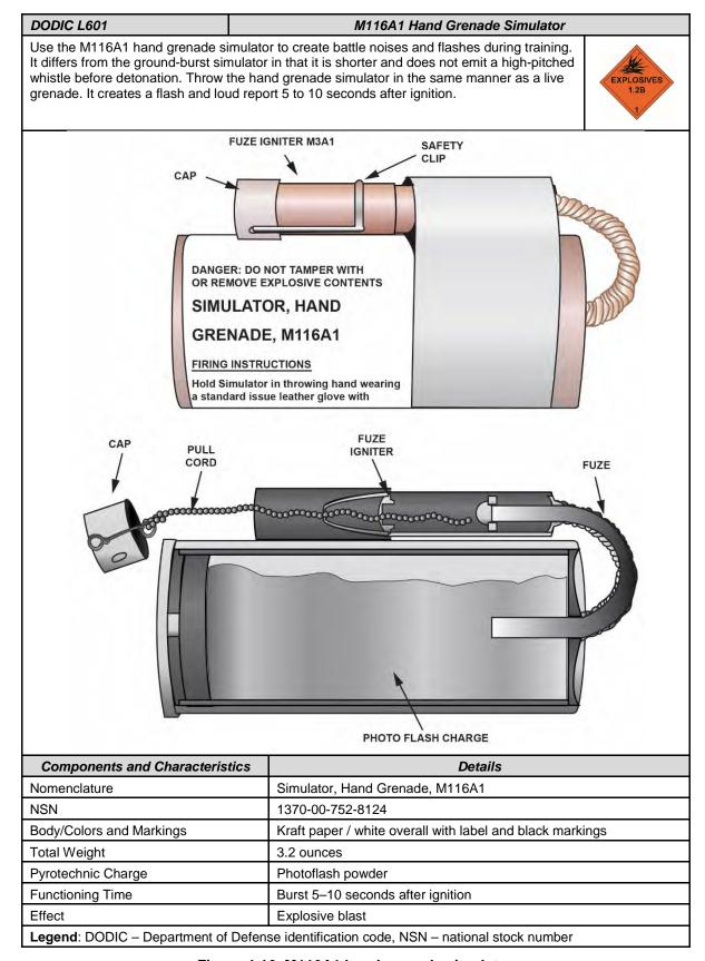
Figure 4-16. M116A1 hand grenade simulator
