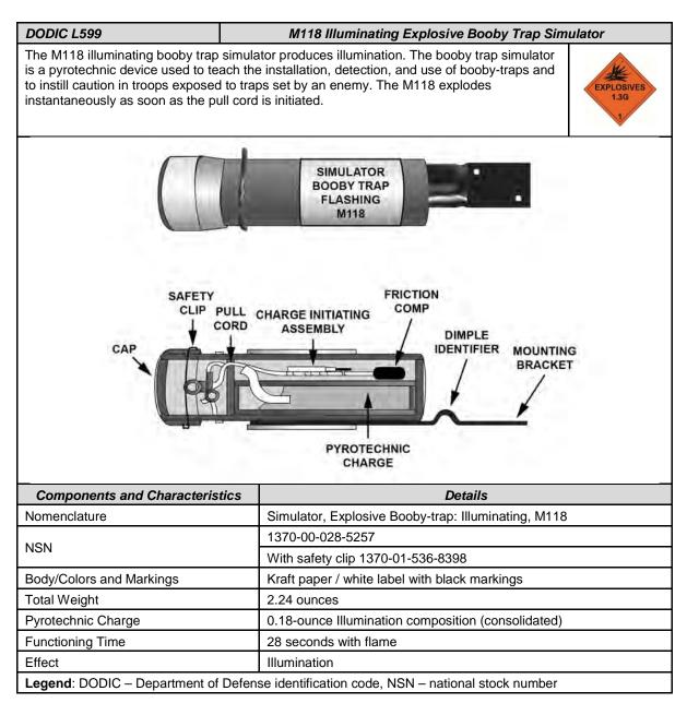
Figure 4-12. M118 illuminating explosive booby trap simulator
