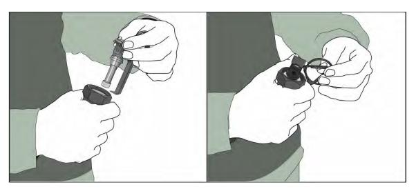
Figure 3-14. Insert the M240 TPF into the M102 body
