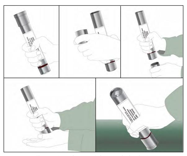
Figure 4-2. Launching pyrotechnic communication signals
