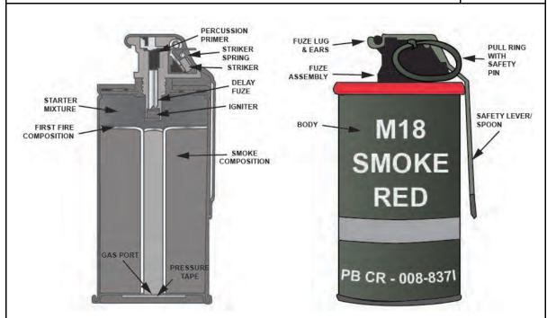
Note. The M18 red is an example of the characteristics of the M18-series smoke grenades.
