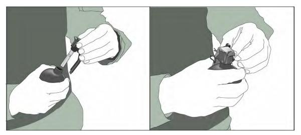
Figure 3-13. Insert the M228 TPF into the M69 TPG body
