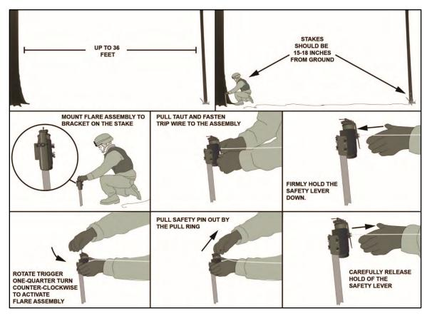
Figure 4-10. Trip flare installation
