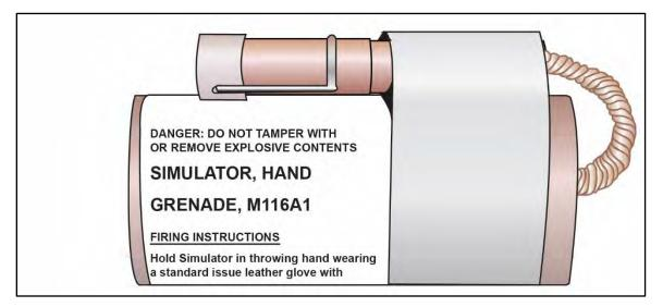
Figure B-15. Hand grenade simulator
