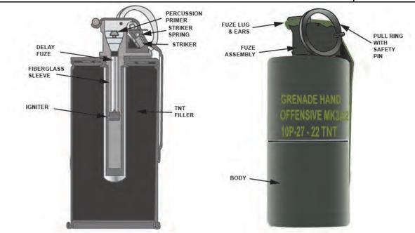
**Note.** The MK3A2 OHG has been found to contain 17–50 percent chrysotile asbestos in the fiber body and is restricted for use in contingency operations only. In case of emergency use, commanders must limit unit personnel exposure to two or fewer MK3-series grenades detonations in an 8-hour period.
