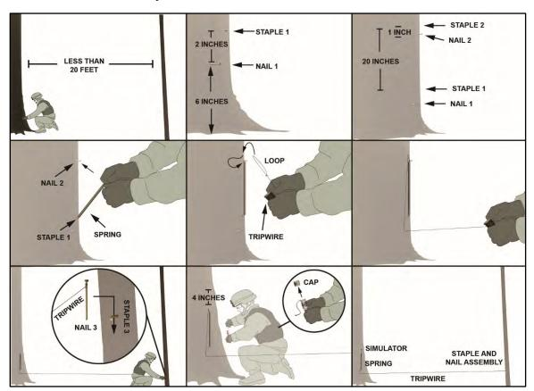
Figure 4-14. Early warning simulators installation
