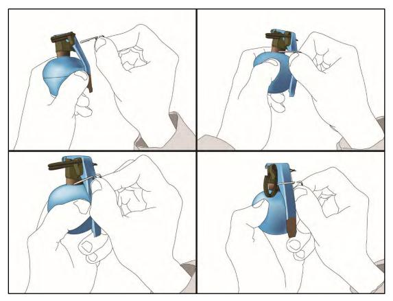
Figure B-4. Safety clip installation
