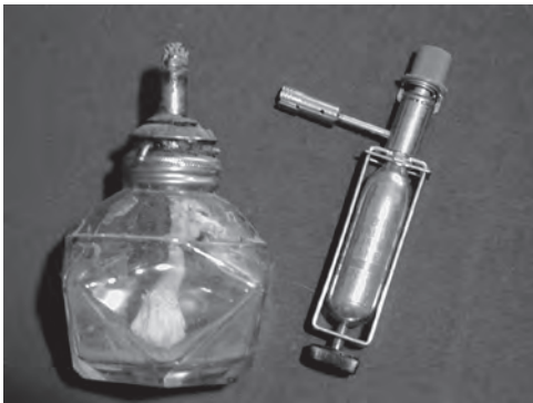
Above: Heat sources Alcohol lamp (L); Butane torch (R)
