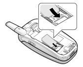
4. To remove the SIM card, slide it upwards, as shown, and take it out of the socket.
