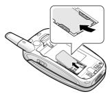
**5.** Replace the battery so that the tabs on the end align with the slots at the bottom of the phone.
