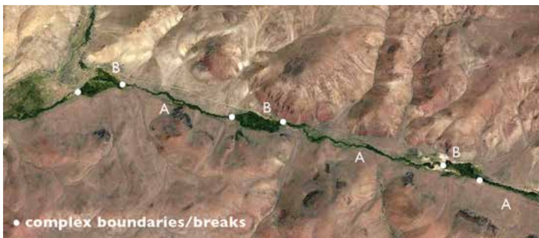
Figure 5. Alternating lotic complexes within a valley segment reflect the influence tributary fans have on the main stream valley. Where fans are wide and dominate the valley floor, the riparian corridor is “pinched” and narrow (complex A). Upstream of fans, the valley bottom is locally flattened, allowing a broader expression of riparian communities (complex B). Streamflow is from right to left. (Image obtained from Esri World Image Service. World_Imagery - Source: Esri, i-cubed, USDA, USGS, AEX, GeoEye, Getmapping, AeroGRID, IGN, IGP, and the GIS User Community.)
