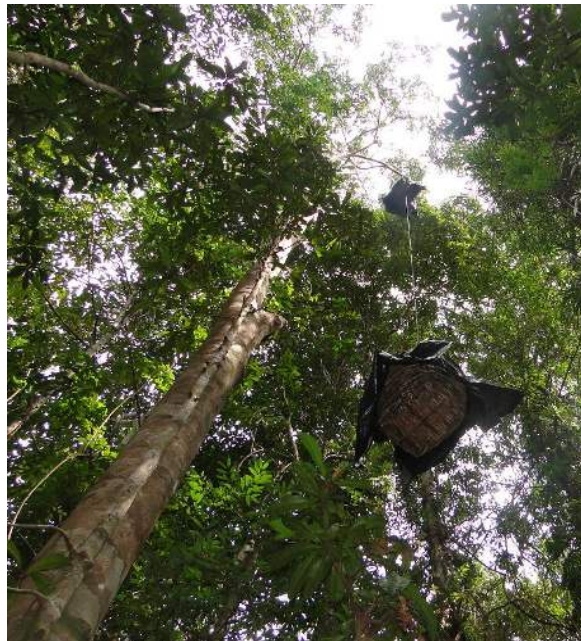
Fig. 2-7: Test set-up for height tests Measurements at 5m and 15m; the black plastic cover on top of the wooden baskets protected the batteries of the traps from heavy rainfall.
