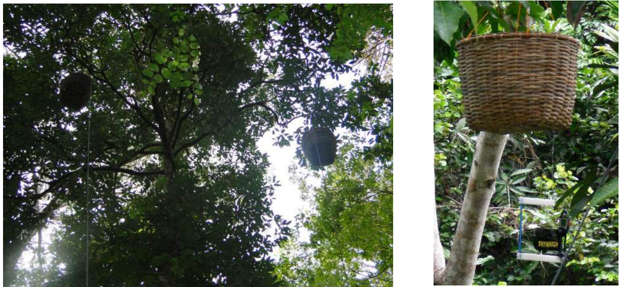
Fig. 2-6: Test set-up for exposure tests Left: The two traps at J25, with the unexposed trap on the left side and the exposed trap on the right side. Right: The SKYWATCH-device was attached to the bottom of the wooden basket.
