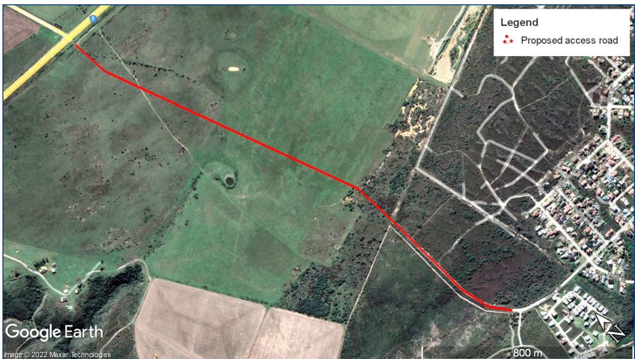
Figure 1-2: Aerial photograph of proposed new access road.
