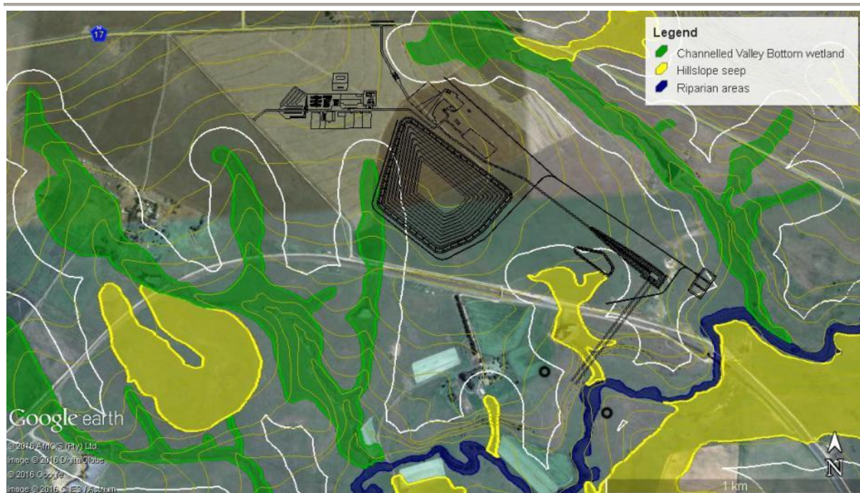
Figure 40. A more detailed illustration of the proposed aboveground mining infrastructure (indicated by the black lines) in relation to the delineated wetlands (as per the legend). The 100 m buffer is indicated by the white lines and the contours by the orange lines.
