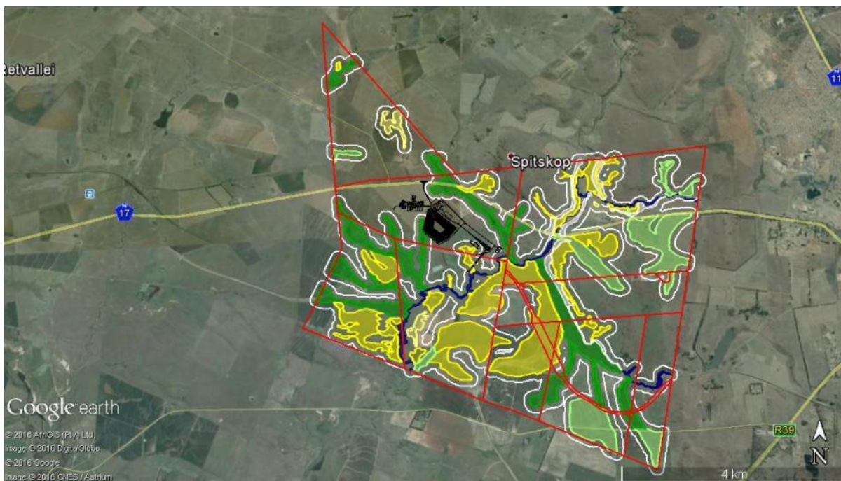
Figure 39. The proposed aboveground mining infrastructure in relation to the delineated wetlands and the 100 m buffer (as indicated by white lines).
