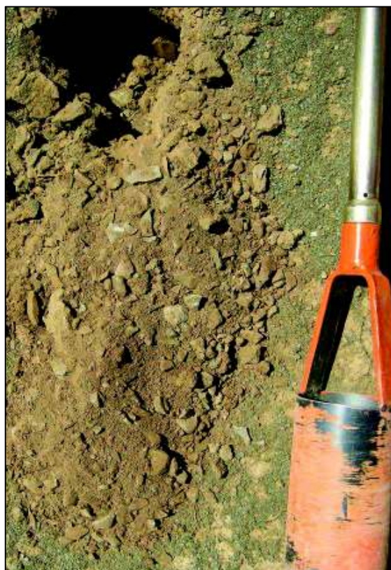
Figure 16: An example of a shallow Glenrosa encountered in the De Aar area
