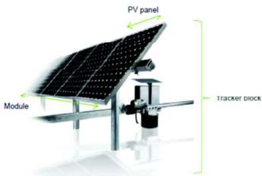
Figure 9: Single axis tracking system (image courtesy of Mulilo)
