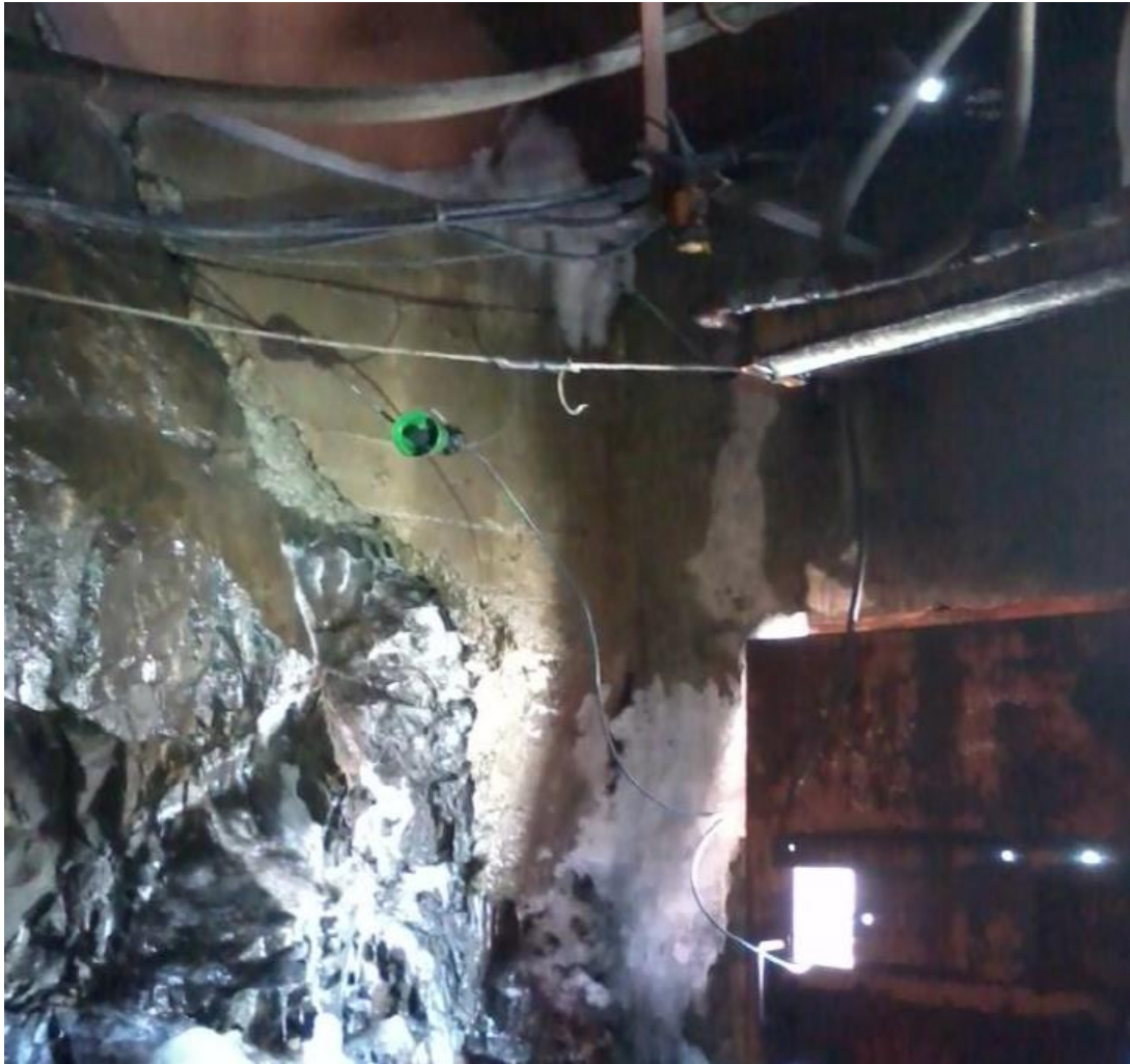
Figure 2-1 Unidirectional microphone inside adit door.
