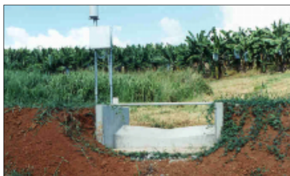
Runoff weir on a banana farm. (Photo: Cardwell Shire Catchment Management Association)
