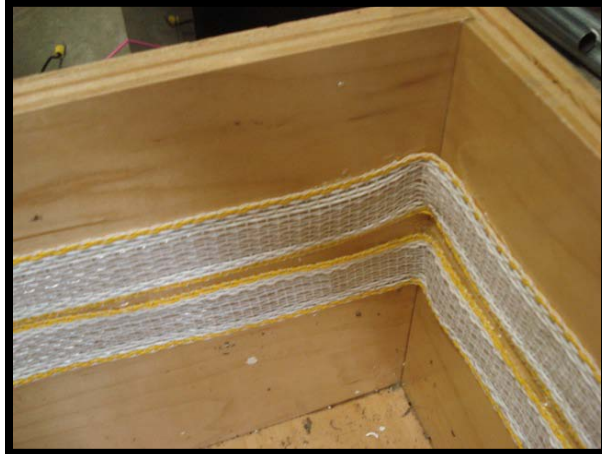
Livestock tapes mounted in test box
