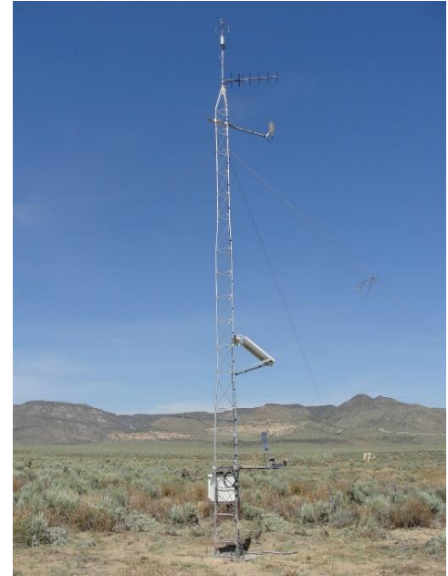
Figure A-13. Example of a typical MEDA station with a 10-meter tower
