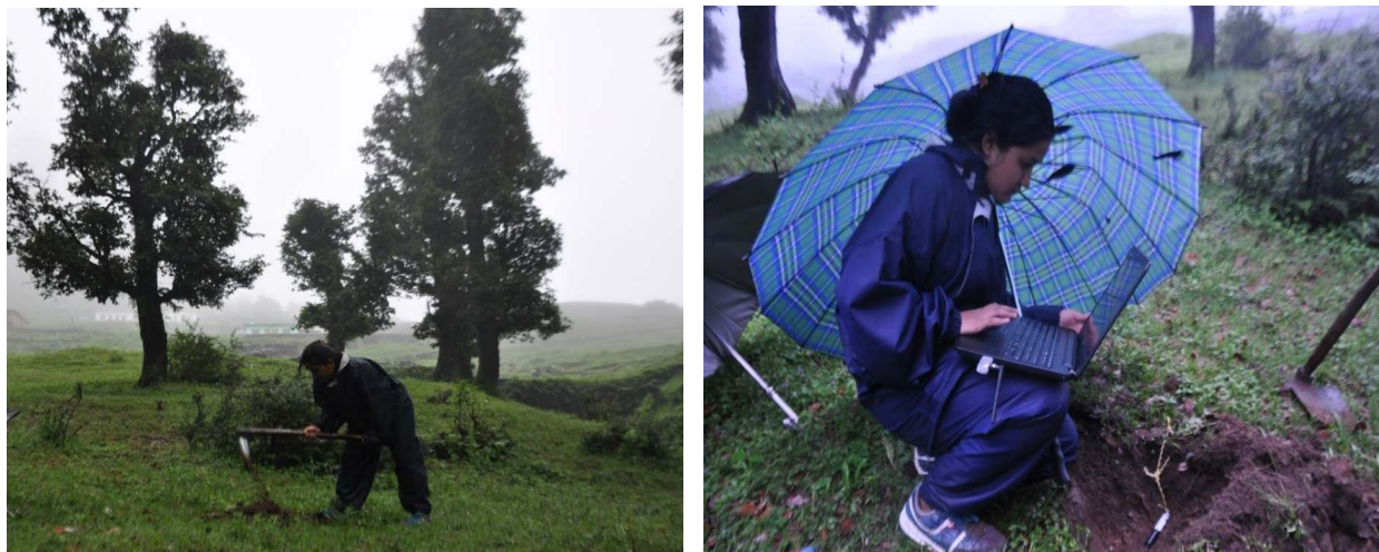
Fig. 7: Installation of soil data loggers in study transect
