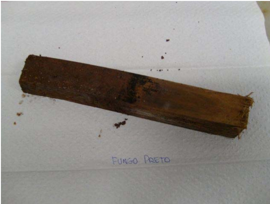
Figure 2 – Aspect of bamboo strip after 15 days of exposition.
