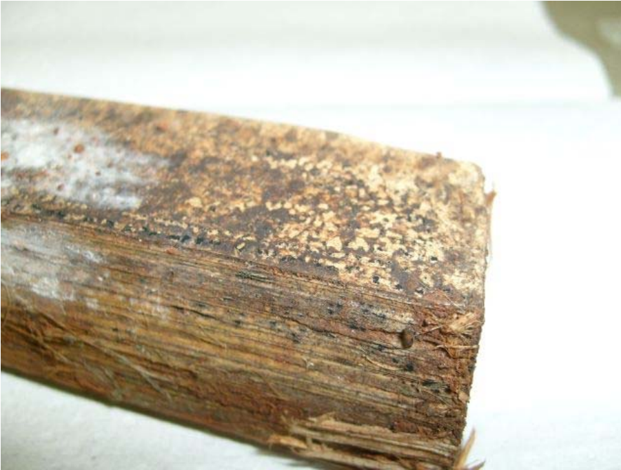
Figure 3 – Fungi spores (dark spots) and mycelia (white areas) infesting bamboo.
