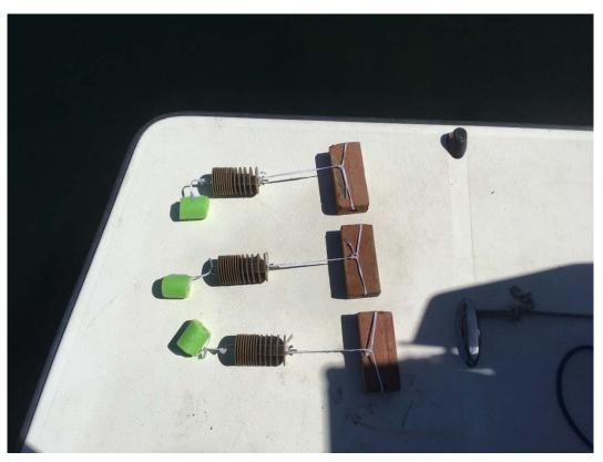
Figure 4. EPA Hester-Dendy Artificial Substrates for aquatic macroinvertebrate sampling.
