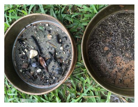
Two standard sieves used to sort petite Ponar benthic samples with sieve #10 (2 mm) on left and sieve #30 (500 micron) on right.
