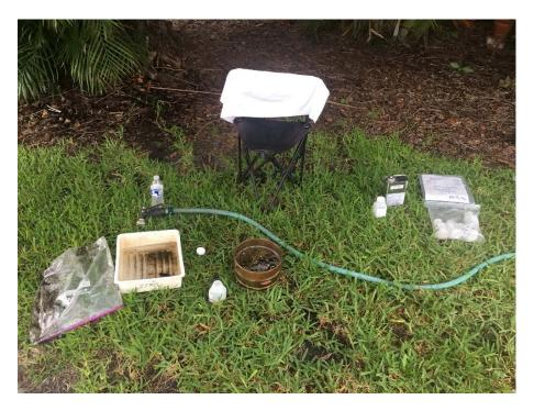
Ponar Sample processing and preservation station using standard serves to sort benthic macroinvertebrates from sediments and debris.
