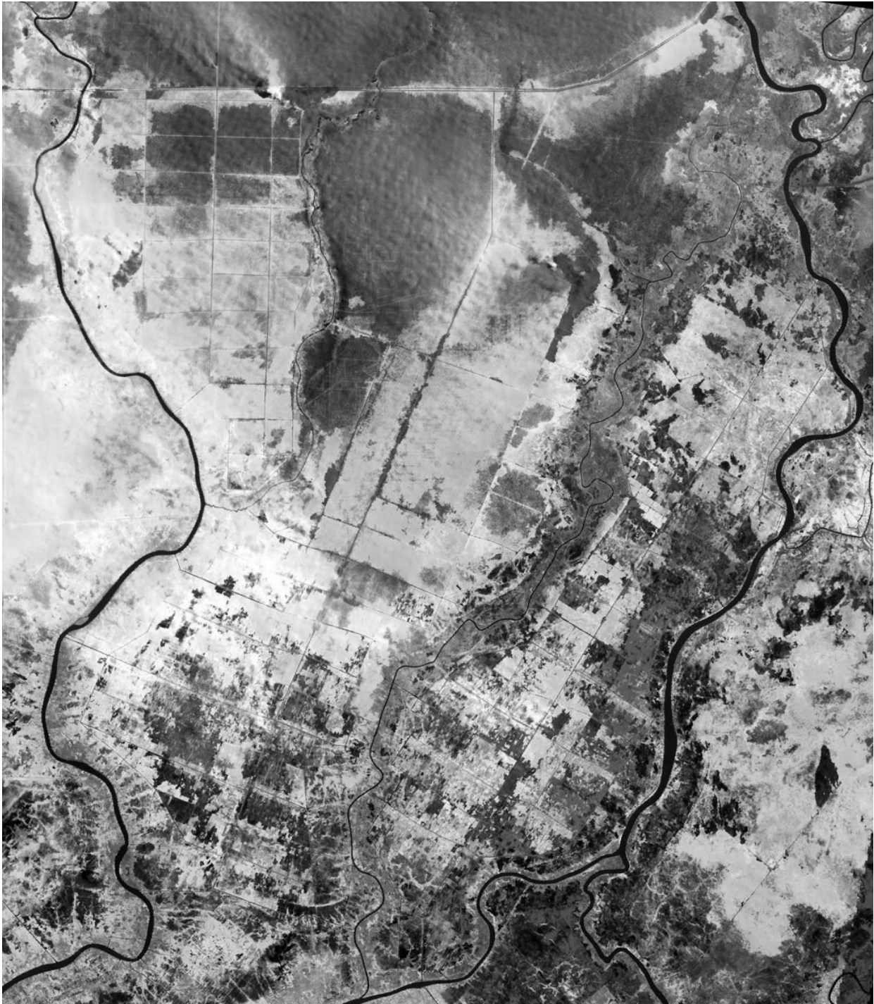
Figure 17. Landsat image (118-62, RGB=543) acquired on 20. Aug. 2001 from the MRP area located between Kapuas (left) and Barito rivers (right) with Lamunti and Dadahup villages. The time of acquiring the image is again during dry season visible with smoke plumes four years after the ENSO of 1997 and one year before ENSO 2002. The MRP channel system can be seen and it is mostly not working. The clear cuts of the peatland is shown in light green colour with regrowth of bush land. Red colours around the channels are burnt cars and fresh clear cuts, compare Fig. 2, 9A,C+F, and 11. The remaining PSF (dark green colour) in the upper part of the image is strongly reduced see Figure 2.
