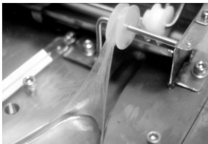
Figure 4. Direct filament preparation of BC by shallow pan
