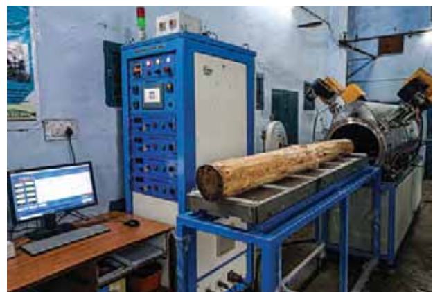
Microwave Vacuum dryer for wood drying
