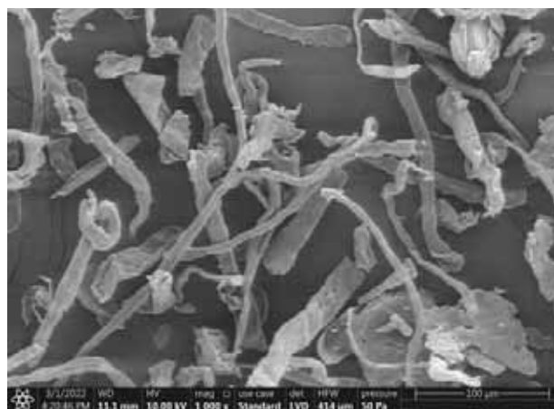
Micrograph of Bamboo Cellulose Nanofibrils produced by Cryo-crushing
