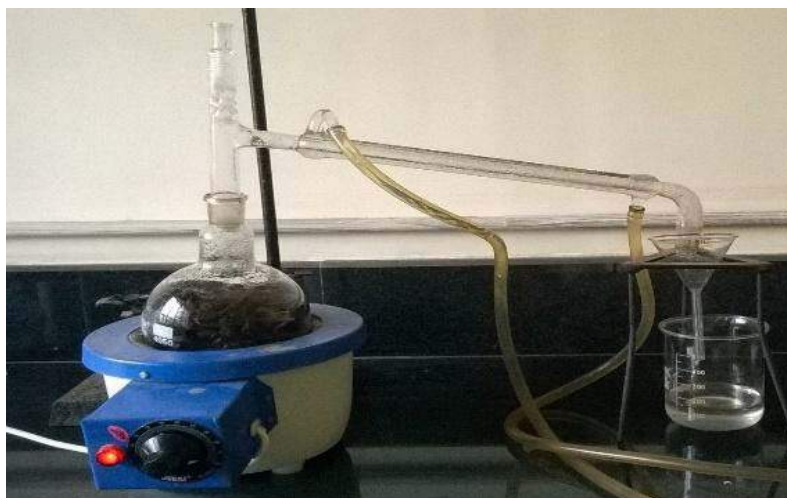
Figure 2: Extraction of cinnamon oil from whole dried cinnamon barks using distillation flask.
