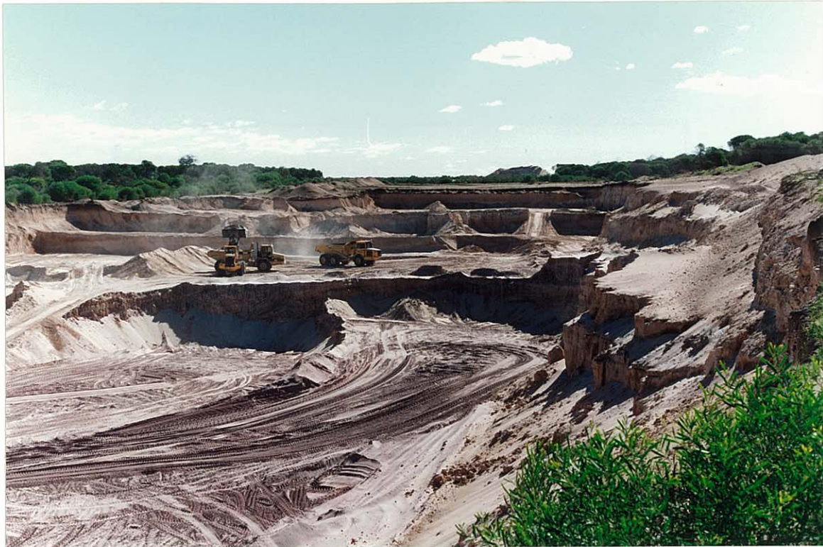
View looking North - West along mining direction showing ore face and overburden benches in the main pit.
