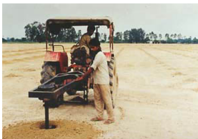
Fig. 1. Auger-hole technique for planting trees in alkali soil.
