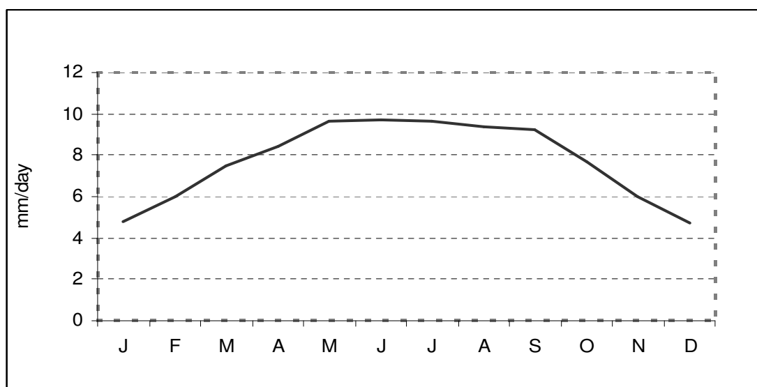
Figure 1.8. Average monthly evaporation for Sayun. It ranges between 4.5 to 6 mm/day in winter, and between 7.5 to 9.7 mm/day during the spring and summer.
