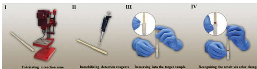
Fig. 6 Schematic of the fabrication process of LADs: (I) fabrication of a reaction zone; (II) immobilization of the colorimetric reagents; (III) immersion of the LAD into the target sample; (IV) colorimetric recognition of the results into the reaction zone. Reprinted with Creative Commons CC BY license [7]
