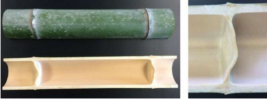
Fig. 3 Left: Segment of a bamboo culm. Right: Magnified view of the section near a diaphragm. Reprinted with permission from [20], Copyright 2016, American Physics Society
